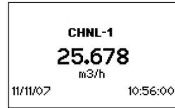
The main measurement unit is displayed when first entering the measurement screen. Press **MUX** to switch between channels 1 and 2. Press **NEXT** to cycle through the three line display, totaliser and dual measurement screens.
