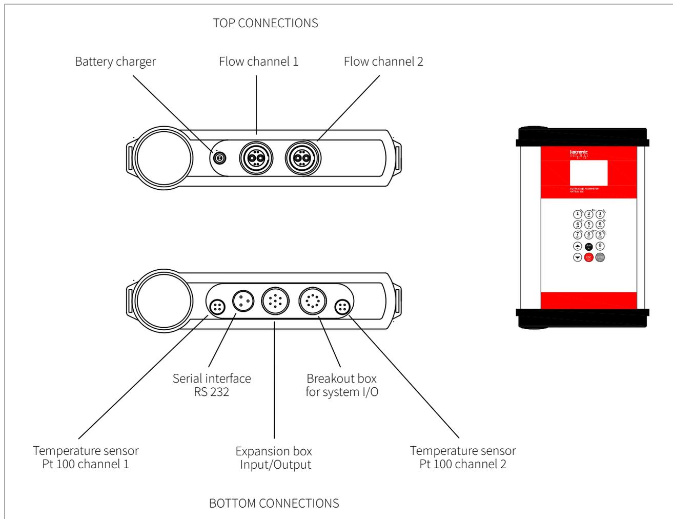
Picture 8: Electrical connection diagram KATflow 230
