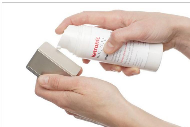
Picture 9: Application of acoustic coupling gel
