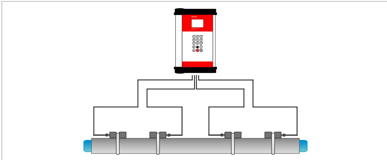
Picture 3: KATflow 230 in a 1-pipe 2-path configuration
