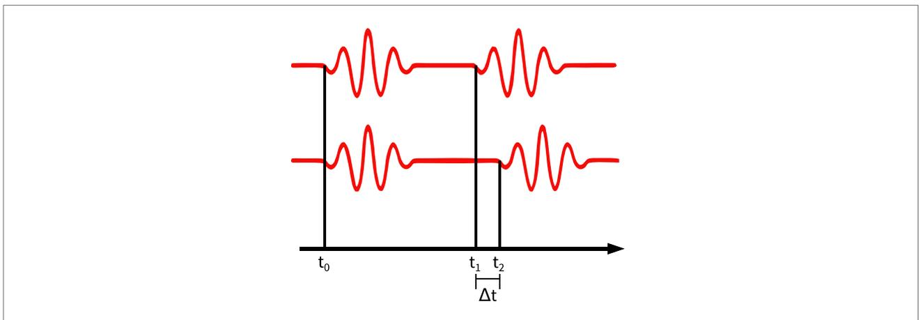
Picture 2: Transit-time measuring principle
