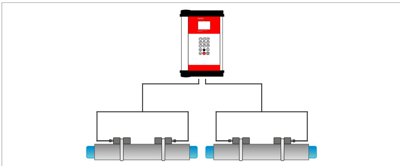
Picture 4: KATflow 230 in a 2-pipe 1-path configuration
