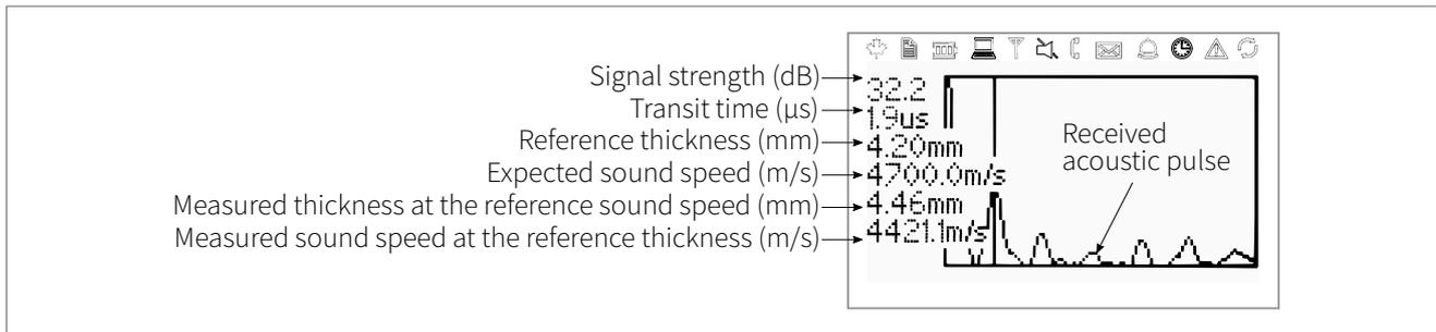
Picture 19: Wall Thickness Gauge (WTG) screen
