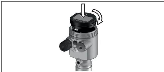
Fig. 27: Installing the display and adjustment module in the electronics compartment of the single chamber housing
