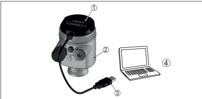
Fig. 35: Connection of the PC via VEGACONNECT and USB
