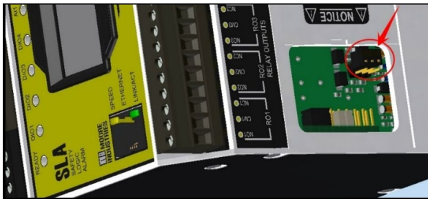
Figure 4.11 Relay 4 jumper moved to the stowed position, changing relay to a process relay.
