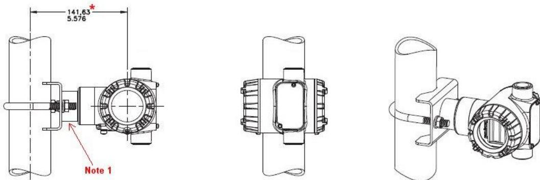
**VERTICAL FLAT PIPE MOUNT****Figure 6 – STT750 Pipe Mount with adapter housing - Horizontal & Vertical**
