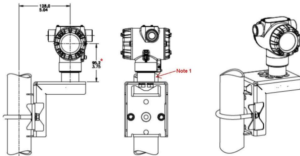
**VERTICAL ANGLE PIPE MOUNT****Figure 7 – STT750 Pipe Mount, Vertical**
