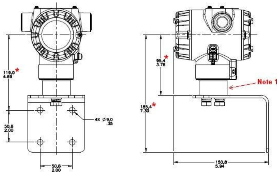
Figure 4 – STT750 with adapter housing - Horizontal Wall Mounting
