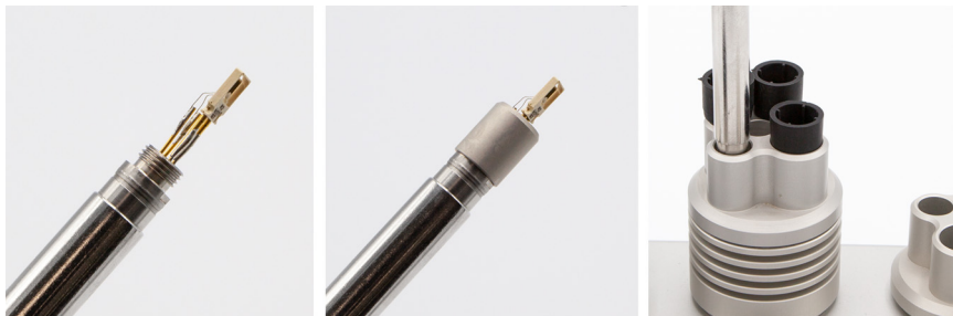
Figure 39 HMP5 calibration with HMK15 using 211302SP adapter
