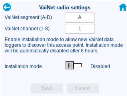
Figure 7 VaiNet segment setting in the AP10 touch interface
