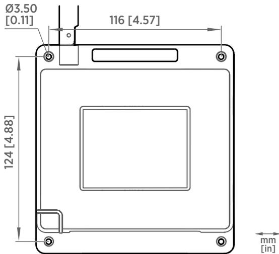
Figure 11 AP10 screw mounting dimensions
