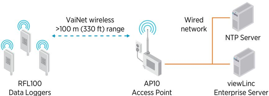
Figure 1 AP10 in the viewLinc Monitoring System
