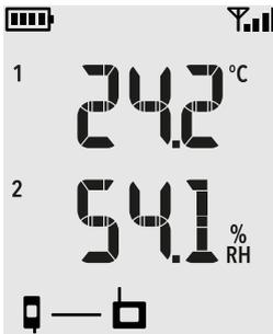
**Connected to an access point but viewLinc Enterprise Server not discovered yet:** Signal strength indicator shows the strength of the access point connection.
