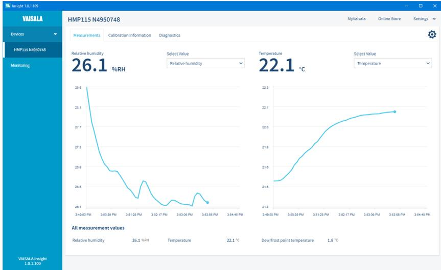
Figure 22 HMP115 probe in Insight software
