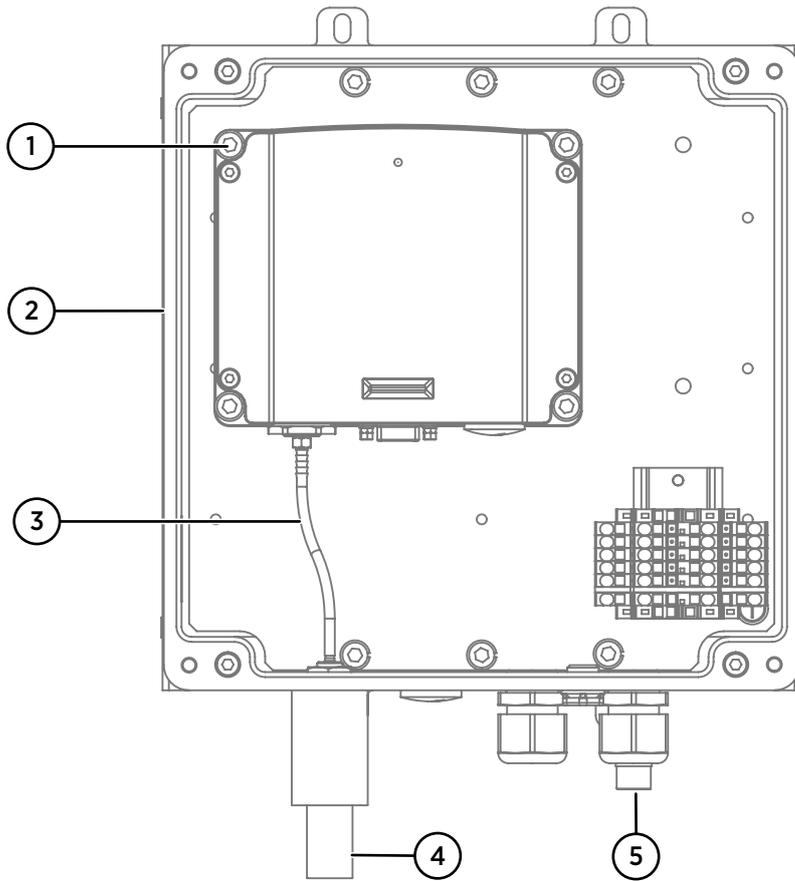
Figure 6 PTB330 inside ASM21113 junction box
