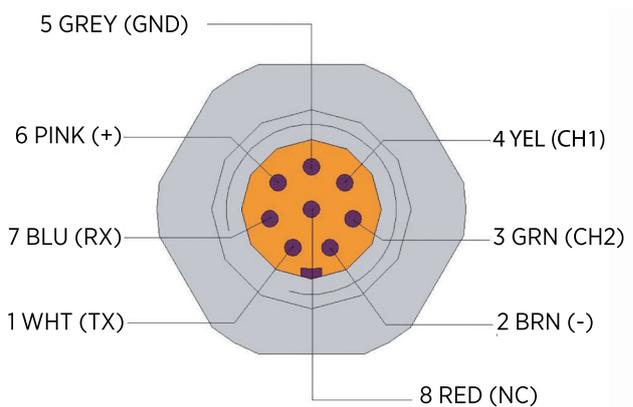
Figure 10 Wiring of optional M12 (8-pin) connector
