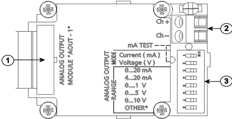
Figure 15 Analog output 1 module AOUT-1T
