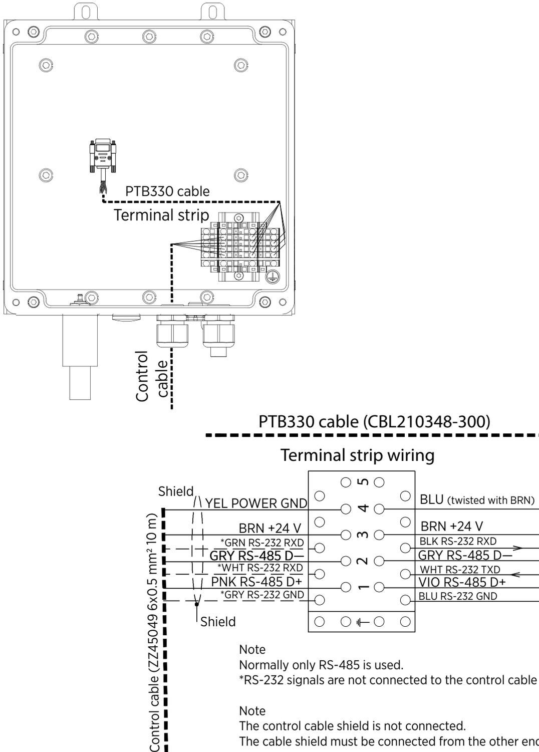
Figure 7 Wiring junction box ASM211113
