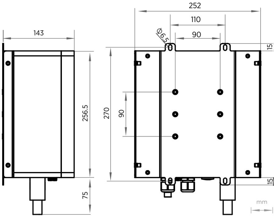
Figure 38 Junction box ASM211113
