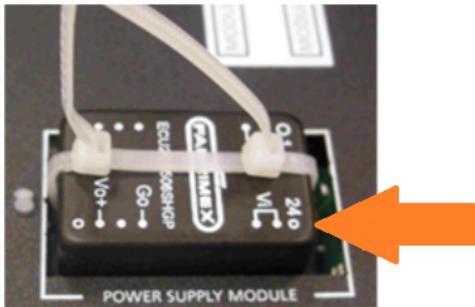
Figure 14 Galvanic isolation module
