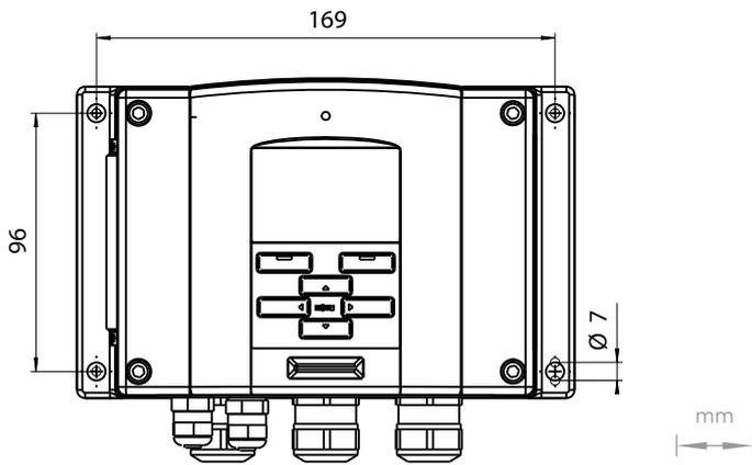
Figure 35 Standard mounting
