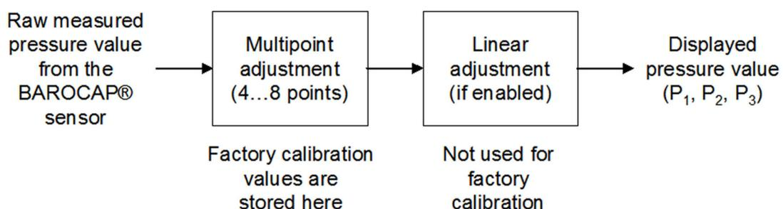
Figure 32 PTB330 adjustments
