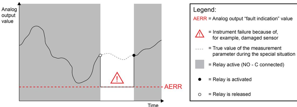
Figure 30 FAULT STATUS relay output mode
