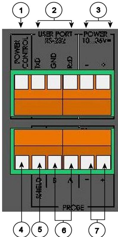
Figure 9 Screw terminal block on motherboard
