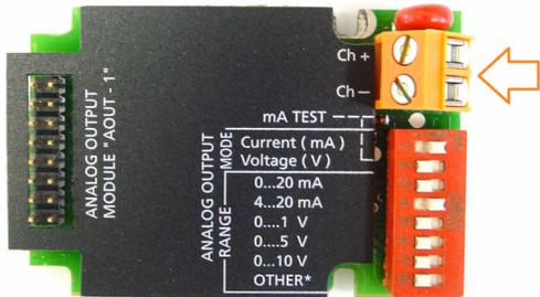
6. Select the current/voltage output by setting **ON** either of the switches 1 or 2.
