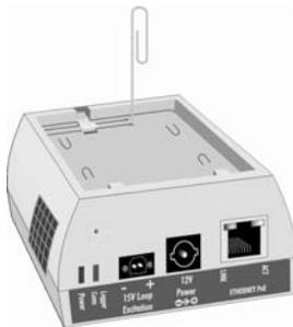
Figure 3: Restart button on vNet Device
