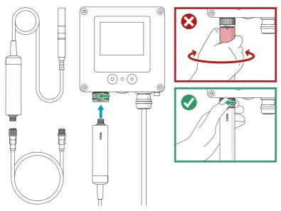
Figure 18 Connecting probe to Indigo300 transmitter
