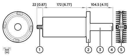
Figure 9 DMP246CS Cooling Set without mounting flange
