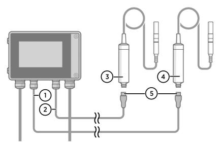
Figure 19 Connecting probes to Indigo500 transmitter
