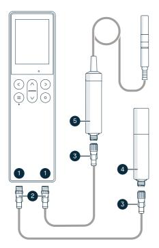
Figure 21 Example of connecting probes to Indigo80
