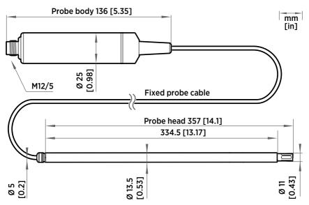
Figure 5 DMP6 probe dimensions
