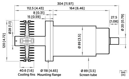
Figure 6 Cooling Set DMP246CS dimensions
