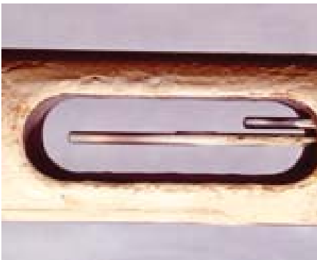
This photo shows the Velocity Sensor Window and Sensor Element remains clean and free of ash buildup. Thereby, Sensor/System performance is maintained and downtime for maintenance is virtually eliminated.
