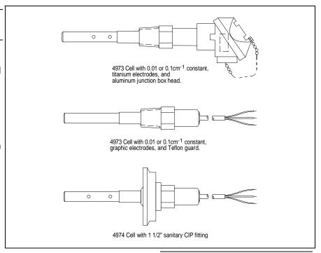
For sanitary clean-in-place (CIP) piping systems, the 4974 cells include standard 1 1/2" or 2" CIP fittings suitable for food and beverage, pharmaceutical and cosmetic, or biotechnology industries. There is no equivalent DL4000 Series for the style of cell.
