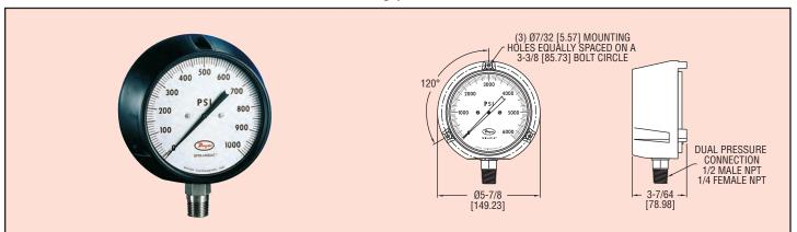
Series 7000B Spirahelic® Direct Drive Pressure Gages with turret mount housings feature a triple coil spiral/helical wound Bourdon tube to provide dependable service. Bourdon tube design eliminates gears, springs, linkages and complex movements which can wear and cause inaccuracy or early failure. Series 7000B gages come standard with a dual-size 1/2" male NPT and 1/4" female NPT process connection.
