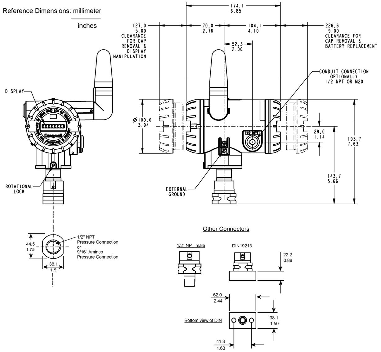
Figure 3a Typical mounting dimensions for in-line models
