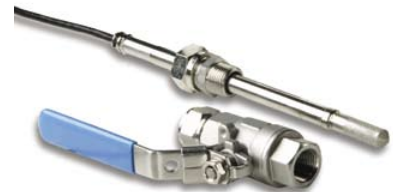
The DMT348 is ideal for installations in pressurized processes where the probe needs to be removed while the process is running. The probe depth is adjustable.
