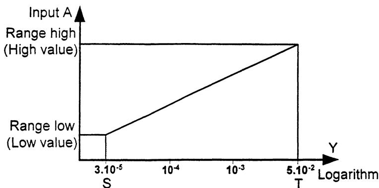
A typical application would be vacuum pressure measurement.
