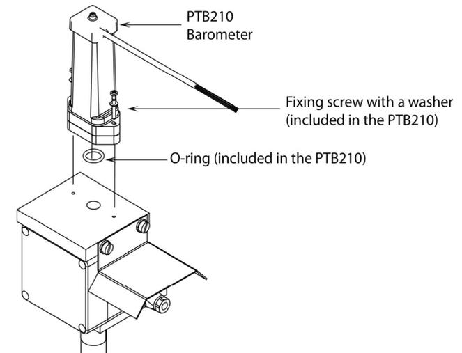
Figure 2 PTB210 Barometer Connection
