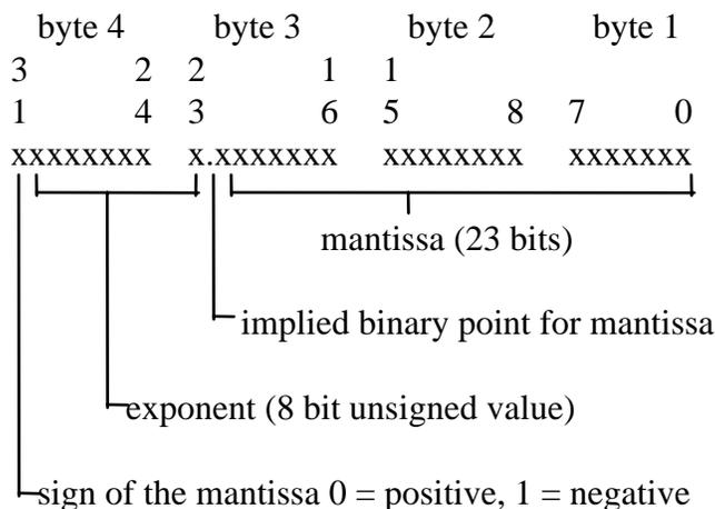
Figure 6-1 IEEE Floating Point Data format
