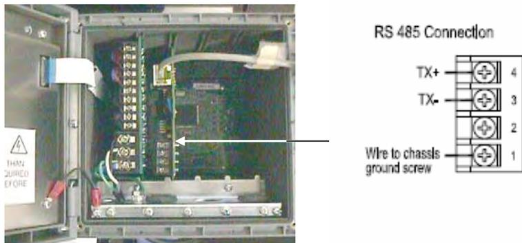
**Figure 2-3 Serial Port Wiring**
