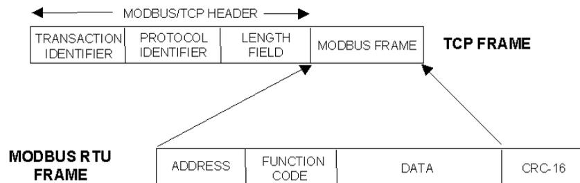
**Figure 5-1 Modbus RTU Protocol within a TCP/IP Frame**
