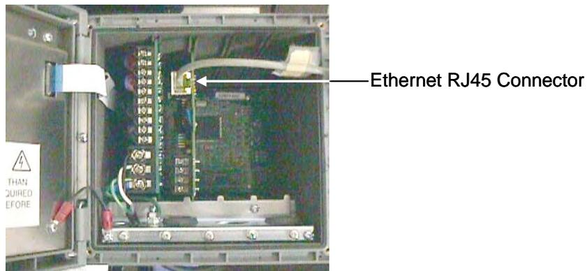
Figure 2-2 Ethernet Port Wiring
