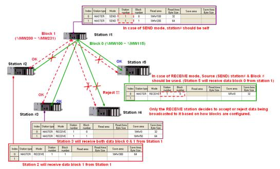
High Speed Link (HSL) services in Fast Ethernet module (FEnet) ensures efficient and reliable peer-to-peer networking of MasterLogic-200 PLCs.
