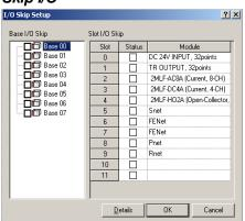
Skip I/O setting for any base/slot module instructs the CPU to skip processing of specified I/O module(s). The input image (%I) area would not be refreshed for those modules and output image area will not be transferred to the actual module.
