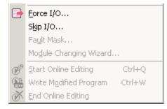
Any part of the PLC program can be edited online when CPU is running & the new program can be downloaded to the CPU without having to stop the CPU.
