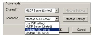
The Snet module can be configured to serve open standard MODBUS RTU or ASCII slave protocol for allowing any third-party controllers / HMI / SCADA to communicate with MasterLogic PLCs.
