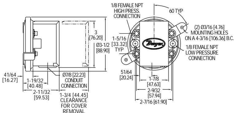
Series 1910 pressure switch. All pressure and electrical connections and set point adjustments are on one side for easy installation.
