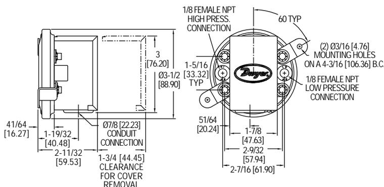
The Dwyer-engineered force-motion amplifier increases the leverage of diaphragm movement and results in a switch with excellent sensitivity and repeatability.
