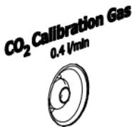
Transmitter models with CO<sub>2</sub> measurement have an inlet for calibration gas. Supply the calibration gas with a known concentration (for example, 1000 ppm) to this inlet using a 3 mm inner diameter silicone tube and a 0.4 l/min flow.
