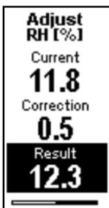
In the adjustment screen, turn the trimmer to set the desired correction. To commit the change, stop turning the trimmer and wait.
