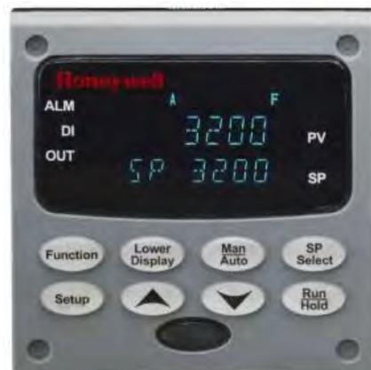
Figure 4-1 Operator Interface
