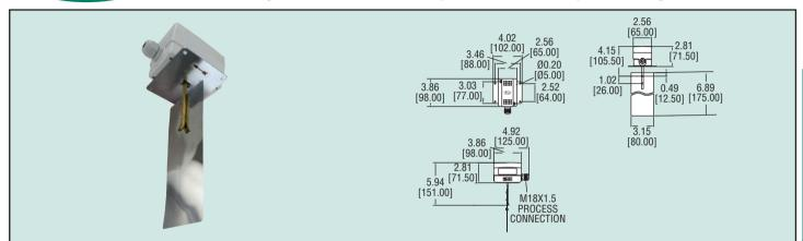
The Model AAFS Adjustable Air Flow Switch is capable of detecting a wide range of air velocities with minimal user calibration. The adjustable screw changes the set point at which the SPDT snap switch engages. Quality features include a stainless steel vane, galvanized steel base, and ABS enclosure. The unit is field adjustable from 200 to 1800 FPM (1 to 9.2 m/sec).
