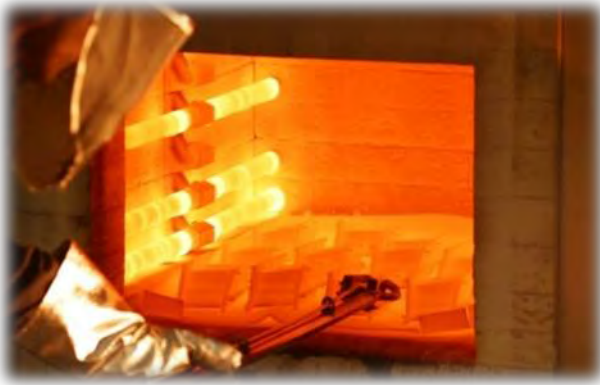
Figure 1. Furnaces used in heat treatment applications require accurate and reliable control system performance.
