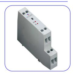
The SEM213/P is a cost effective "smart" DIN rail mount transmitter that accepts resistance temperature sensors and converts sensor output over a configured range to a standard industrial (4 to 20) mA transmission signal.
