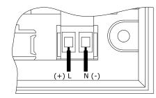
Wires are retained by screws. Ensure that the exposed section of the wire is fully inserted and that no loose strands are exposed.
