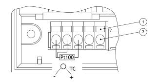
To make a connection: Insert small screwdriver blade into tension clamp orifice, (1) push and twist to deflect clamp into open position. Do not lever screwdriver thus forcing connector body sideways. Insert conductor tail sufficiently into (2) then release screwdriver. Ensure no loose wire strands protrude.
