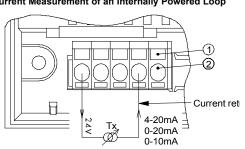
A 24V internal power supply is available to power external field transmitters.
