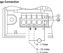
To make a connection: Insert small screwdriver blade into tension clamp orifice, (1) push and twist to deflect clamp into open position. Do not lever screwdriver thus forcing connector body sideways. Insert conductor tail sufficiently into (2) then release screwdriver. Ensure no loose wire strands protrude
