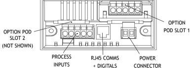
The diagram above shows the rear panel positions for all electrical connections.
