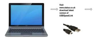
Once software is installed remove protection cover from device port , plug in USB Lead to device ports and connect PC using USB cable.
