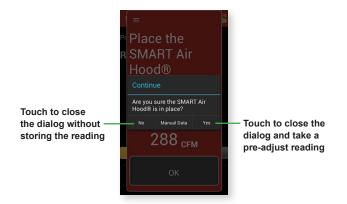
If the **YES** button on the hood placement confirmation dialog was pressed then the app will bring up the Adjust to Target screen.
