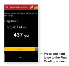
**Note:** Throughout the balancing process the UHH2 can be removed from the pole and taken with you as you balance the branch.
