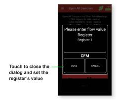
Once all of the registers have been measured, the **NEXT** button at the bottom will become enabled. Press and hold that button until the balance method selection screen appears.
