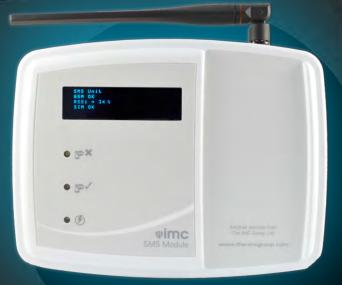
The SMS module uses our own proven protocols. The GSM module has an on-board micro controller acting as watchdog for the system, should any problem with network connectivity be detected the unit will be automatically re-set and re-connected to the network.
