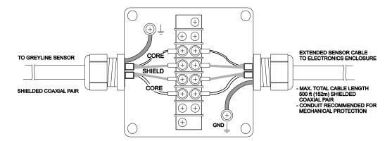
Note: Instead of Micronics Option DXC shielded coaxial pair, you may substitute RG174U coaxial cable from your local electrical cable distributor but this cable is not shielded so extended cable must be installed in metal conduit.
