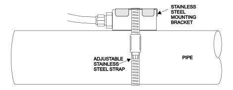
Thread the strap through the bracket and mount loosely on the pipe ready for Sensor coupling.
