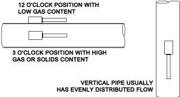
Generally the sensor must be mounted away from flow disturbances such as valves, pumps, orifice plates or venturis which tend to increase flow velocity or cause cavitation. Velocity increasing devices often cause cavitation and erratic operation. As a guideline, mount the sensor 20 diameters upstream and 30 diameters downstream from velocity increasing devices.
