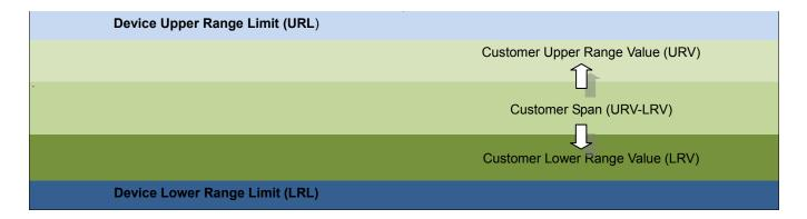
Most manufacturers will supply the necessary data and equations to allow customers to determine these additional errors. Typically, such calculations follow a formula with a form like:
